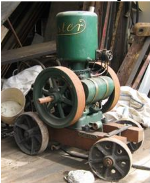
Lister 3.5HP stationary engine
