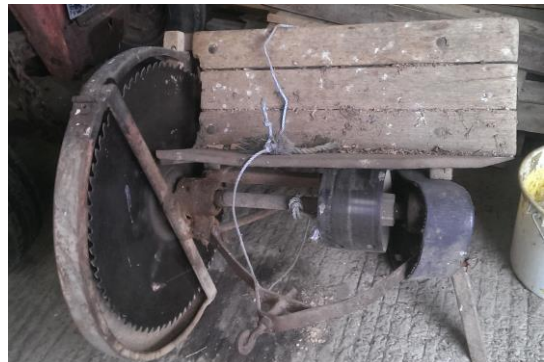
Ferguson saw c/w belt & pulley
