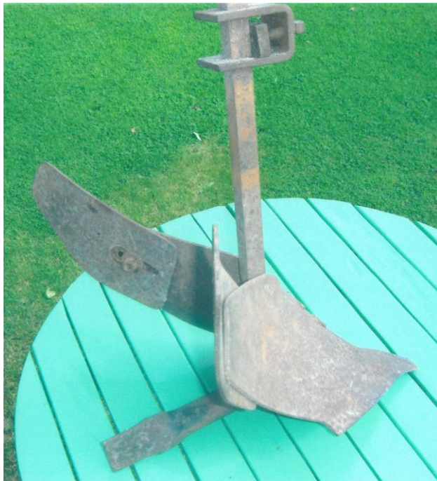
Left - Ridger attachment for garden tractor, possibly Mountfield
